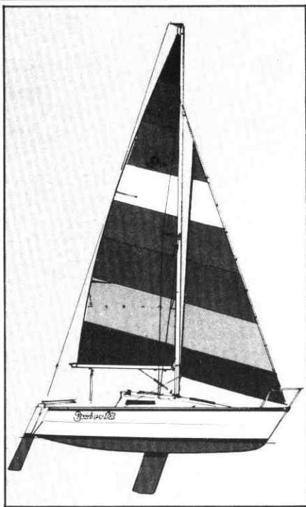
Swift has a high-volume hull, with adequate freeboard, and tall, efficient rig. Her outboard lives in a well, protected by a slide-off cover; quality fittings abound. Note Canpa hatch and extruded alloy toe rail. The keel, which winds up on a screw-jack, kicks up on impact.
